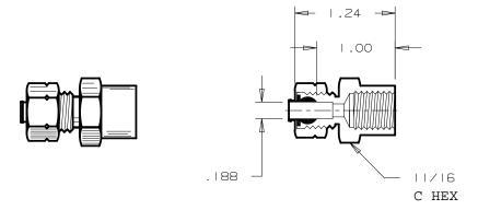
BRASS-FEMALE CONNECTOR, 1/4 TUBE, 1/4 PIPE THREAD, 7/16-24 STRAIGHT THREAD, PARKER BRASS PRODUCTS DIVISION CATALOG PART NO. 66CA-4-4. PRODUCT DESCRIPTION:
