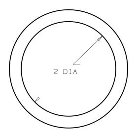
2"I.D. X 3.5"LONG RADIATOR HOSE TO BE CUT TO LENGTH FROM PART NO. 66001564 USE TO CONNECT DASH DIFFUSERS TO HEATER MAIN DUCT ON ALL MVPEF UNITS. [3] REQUIRED PER BUS.
